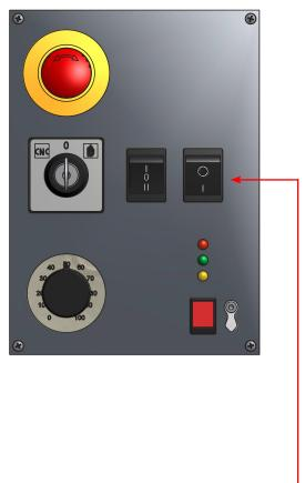
Switch for coolant pump
