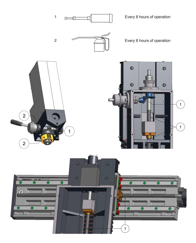
Lubrication of **the drill spindle** and **spindle bearing** is not required, as the ball bearings are closed in by design and are greased for life of the machine at point of manufacture.
