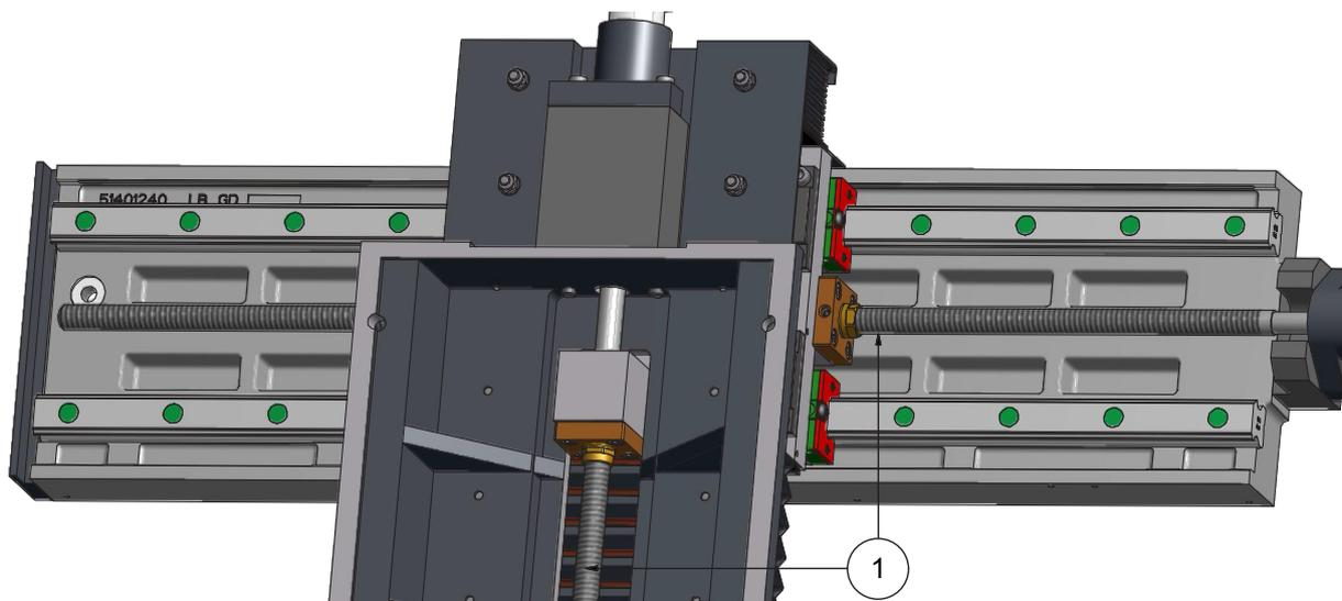
Lubrication of **the drill spindle** and **spindle bearing** is not required, as the ball bearings are closed in by design and are greased for life of the machine at point of manufacture.
