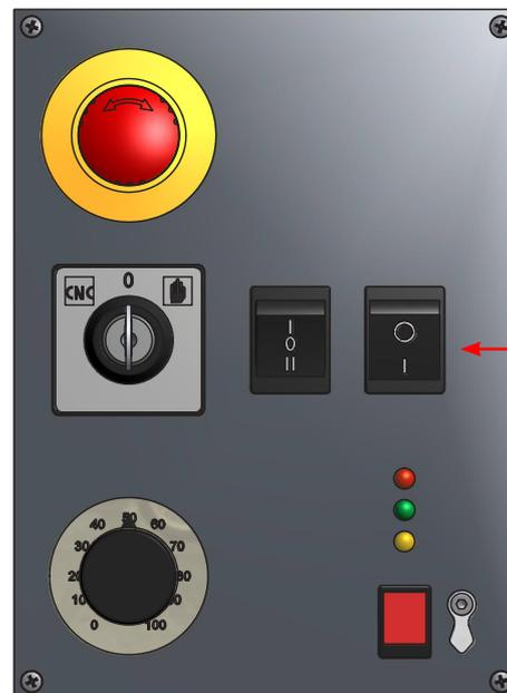
Switch for coolant pump
